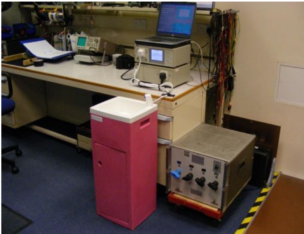
Pic: Voltage Change and Voltage Fluctuations
